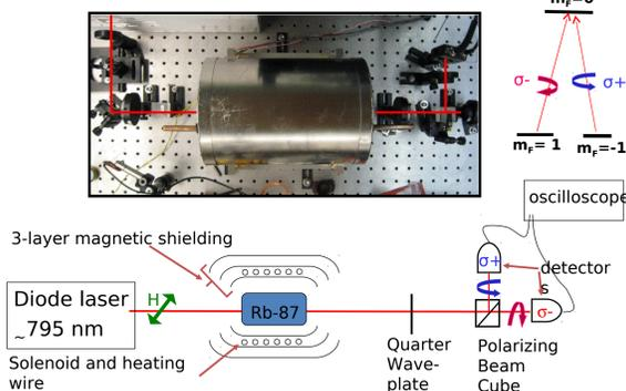
A 795nm laser diode is used to interrogate the isotope, <sup>87</sup>Rb. A cell of <sup>87</sup>Rb and a buffer gas with clear windows at each end of the cylindrical cell to allow for the beam's passage. The cell was magnetically shielded and also encased in a heating apparatus used to take data at different cell temperatures. A quarter
